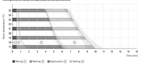
Test conditions: Not pre-chilled vacuum mixing system PALAMIX®, 55 % humidity.
